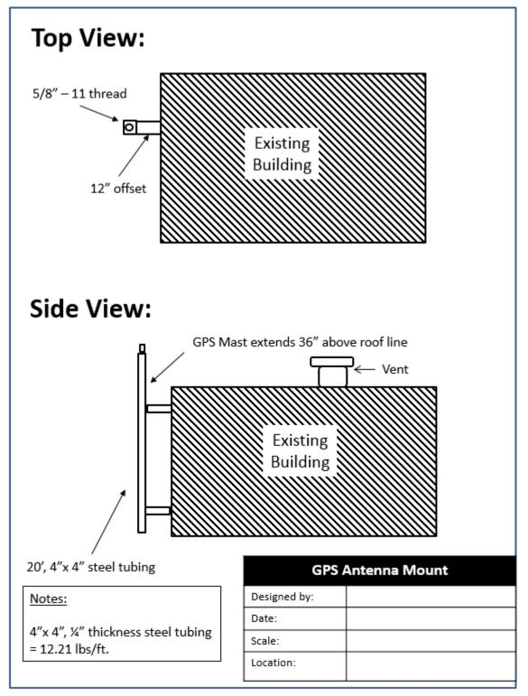
Figure 15: Example Exterior Wall Installation
