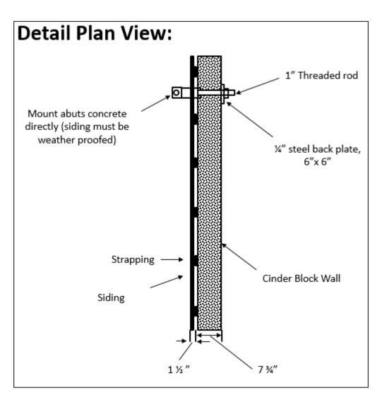
Figure 14: Plan view of an Antenna Mount Installation
