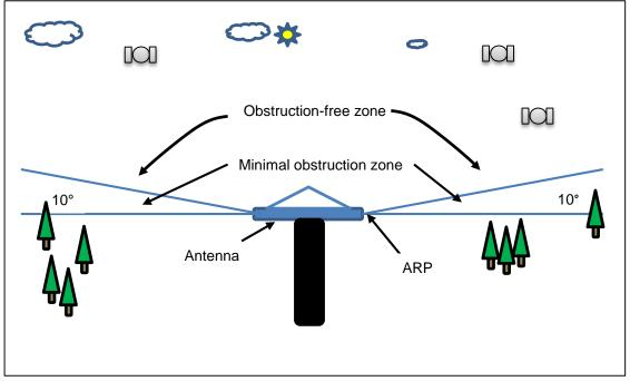
Figure 1: Obstruction-Free Zone around the Antenna
