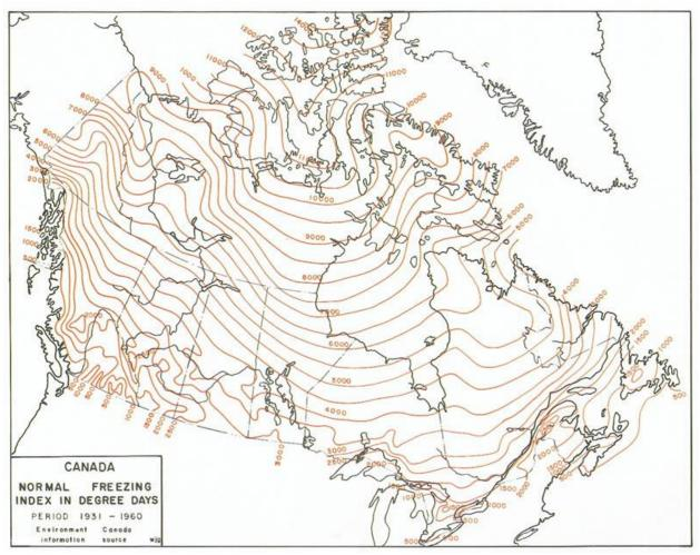
Figure 12: Normal Freezing Index in Degree Days, Canada
