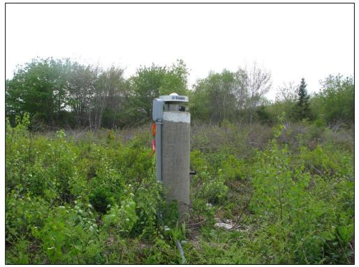
Figure 5: Ground based, concrete pillar monument
