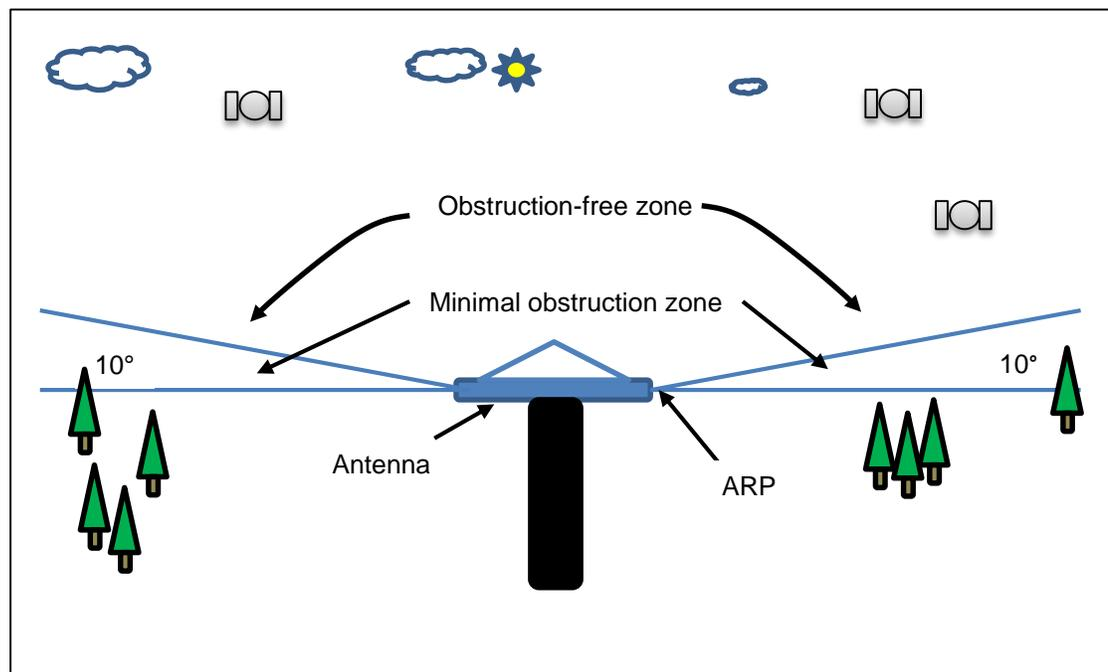
Figure 1: Obstruction-Free Zone around the Antenna
