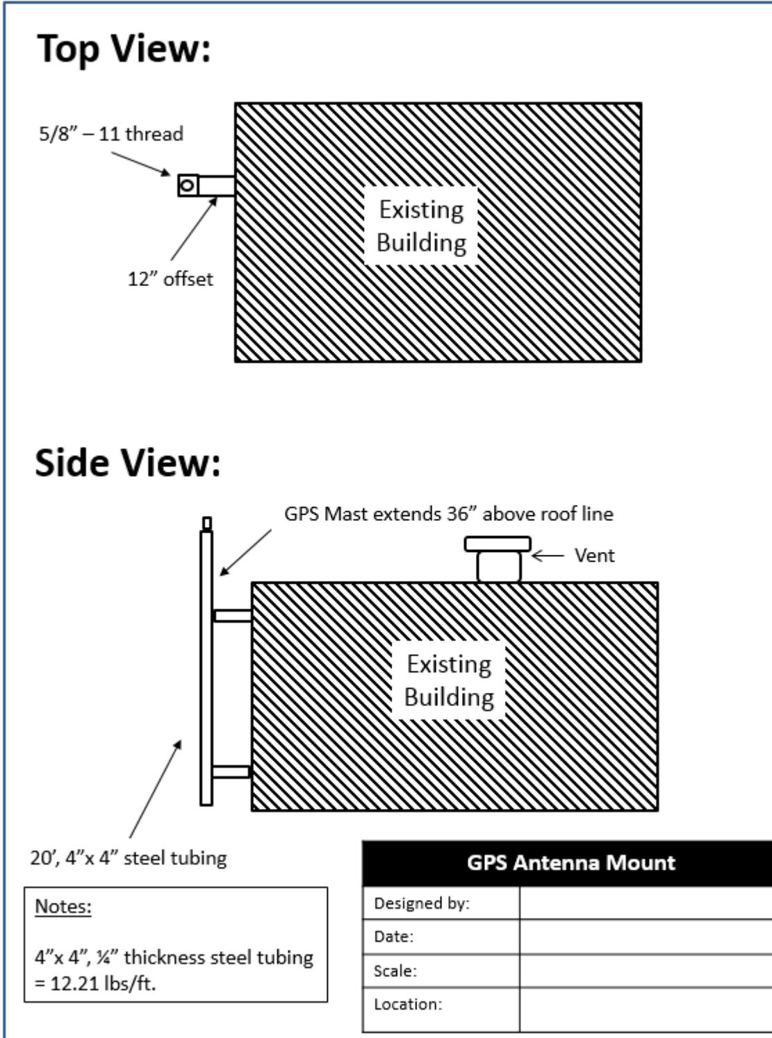
Figure 15: Example Exterior Wall Installation
