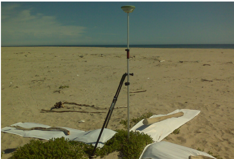
Fig 10 Static GPS Positioning of an Aerial Target on Sable Island.
