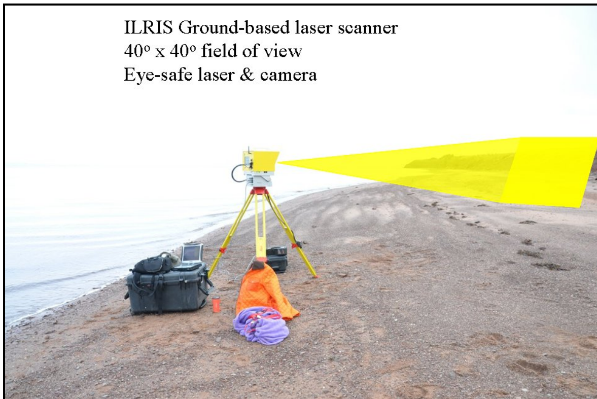
Figure 13 Example of a static lidar system mounted on a tripod to measure the steep slope surface of the coastline.
