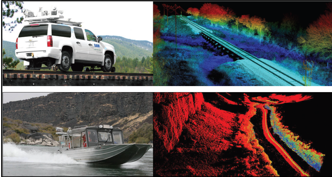
Figure 14 Example of mobile mapping lidar systems. Top photo of a system mounted on a truck on a rail line with associated point cloud. Bottom photo of a system mounted on a boat and associated point cloud. Examples from www.Opech.ca that show the Lynx mobile mapping system from Optech.
