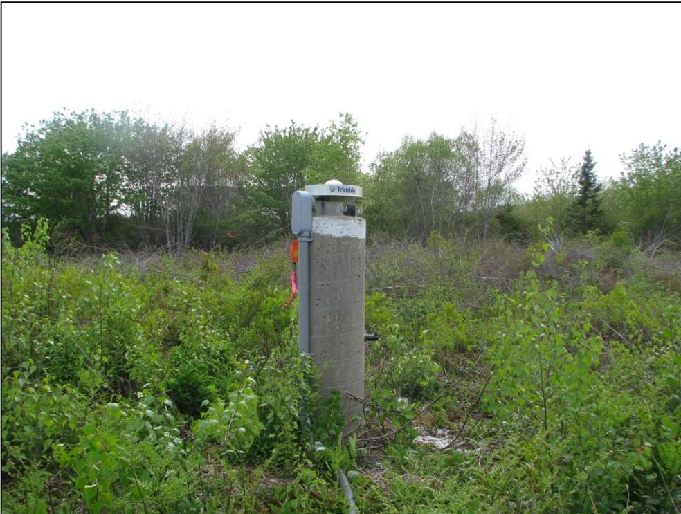
Figure 5: Ground based, concrete pillar monument
